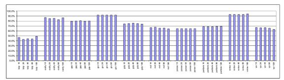
Figure 5: VSBC's miss rate gain with TC in single-threading environment. On average, VSBC is 73.7% better than TC. (Workload = WL0a-j;  $N_{BPC} = 512$ ;  $W_{BBC} = 1$ ).
