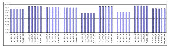
Figure 7: VSBC's miss rate gain with TC in multi-threading environment. On average, VSBC is 85.7% better than TC. (Workload = WL1-9;  $N_{BPC} = 512$ ;  $W_{BBC} = 1$ ).
