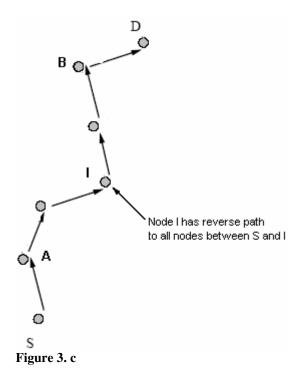
The same way, as the RREP travels back to the source, each node along the reverse path sets up a forward pointer to all nodes along the way to the destination. This is also possible because of the *routers\_list* in RREP (fig3.d).
