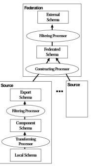
Figure 1: Five-level Architecture for Federated Systems
