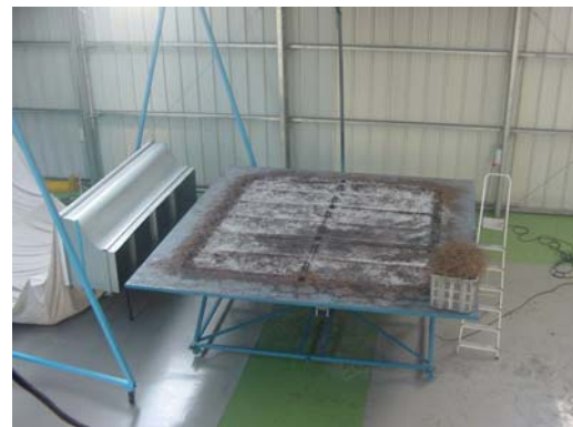
Figure 3: Burn table of 3 \times 3 \text{ m}^2
