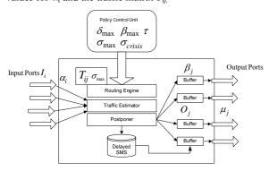
**Figure 4.** Layout of a Typical Gateway Showing its Policy-Driven Control Elements.
