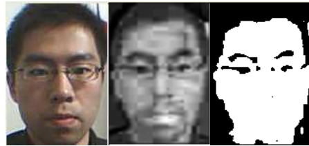
Figure 3. Left: original image. Middle: image based on similarity. Right: binary image
