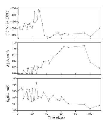
**Figure 8.** Mean values of noise potential, coupling current and noise resistance as a function of time, for paint 4, in 3% NaCl.
