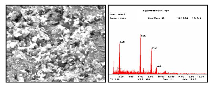
Figure 13. SEM micrograph  $(2500\times)$  and EDAX spectrum of the steel surface after delamination of coating 4 in the electrochemical assay. Electrolyte: 3% NaCl.
