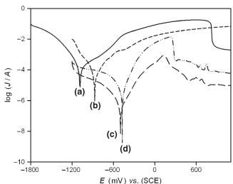
**Figure 3.** Polarization curves of the SAE 1010 steel electrode in the pigments suspensions after 6 h of exposure. Electrolyte: 0.5 M NaClO<sub>4</sub>. Scan rate 3 mV s<sup>-1</sup>. (a) 0.1 M zinc hypophosphite; (b) support electrolyte; (c) 0.1 M zinc hypophosphite + zinc oxide + zinc phosphate and (d) anticorrosive pigment mixture.
