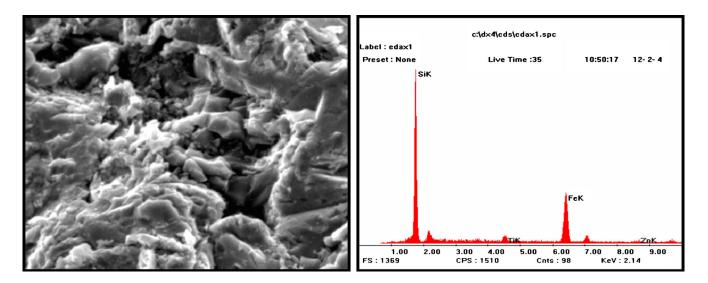
Figure 12. SEM micrograph (2500×) and EDAX spectrum of the steel surface after delamination of coating 6 in the electrochemical assay. Electrolyte: 3% NaCl.
