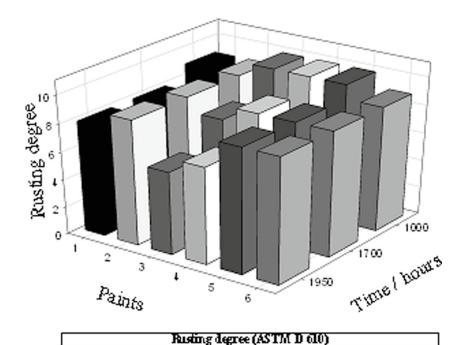
**Figure 4.** Rusting (ASTM D 610) degree of painted panels exposed to the salt spray chamber (ASTM B 117).
