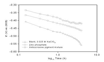
**Figure 1.** Corrosion potential of SAE 1010 steel in pigments suspensions. Electrolyte: 0.025 M NaClO<sub>4</sub>.
