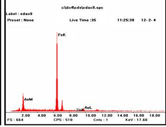
Figure 11. SEM micrograph (2500×) and EDAX spectrum of the steel surface after delamination of coating 2 in the electrochemical assay. Electrolyte: 3% NaCl.
