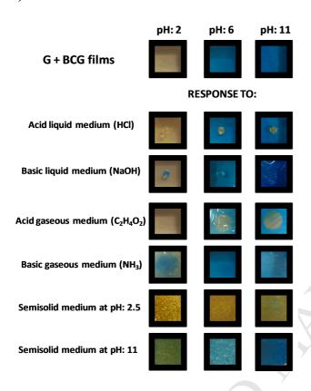
**Figure 3.** Response of gelatin-based films added with methyl orange (G+MO, **A**), neutral red (G+NR, **B**), and bromocresol green (G+BCG, **C**) at pH 2, 6 and 11 after being in contact with liquid, gaseous and semisolid media of different pHs.
