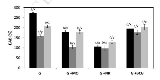
**Figure 4.** Mechanical properties of gelatin-based films obtained at different pH (2, 6 and 11) added or not with different acid-base indicators (MO, NR, and BCG). **A)** Tensile strength (TS). **B)** Young's modulus (EM). **C)** Elongation at break (EAB).
