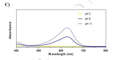
**Figure 2.** Visible absorption spectra (400-800 nm) of gelatin-based films added with methyl orange (**A**), neutral red (**B**) and bromocresol green (**C**) at pH 2, 6, and 11 respectively.
