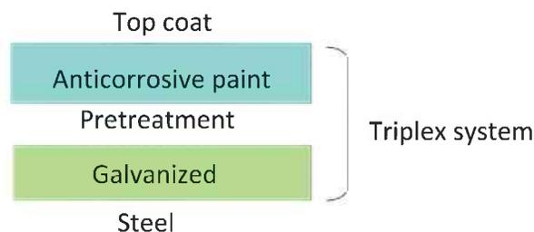
**FIGURE 2** Protection system scheme. [Color figure can be viewed at wileyonlinelibrary.com]
