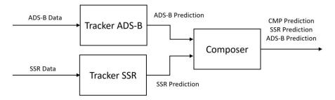
Fig.1: Block Diagram of the Collaboration between Trackers.
