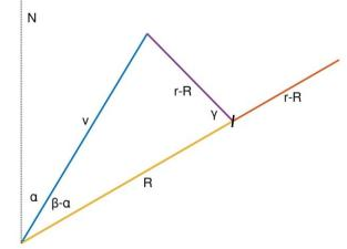
Fig.6: Geometry for calculating the Location of the Reflector.
