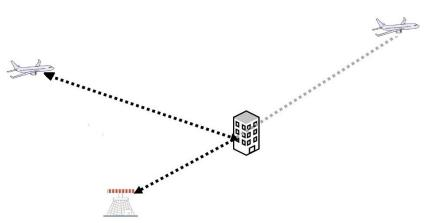
Fig.5: Geometry of Reflections
