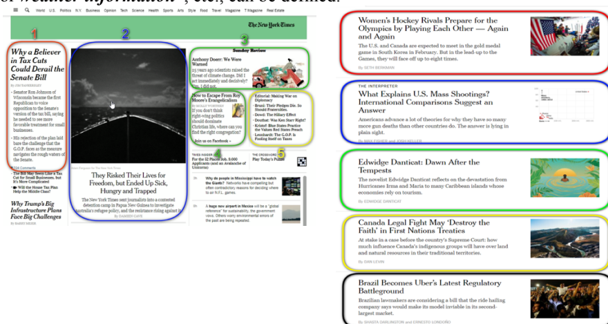
(a) Different parts of the same Web page (b) Sibling elements from the same Web page Fig. 2. Web content blocks: (a) unique items selection (b) sibling items selection.
