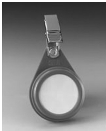
Fig. 1. 3M 3500 monitor used in this study (dimensions: 50 mm \times 30 mm).
