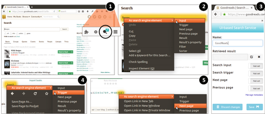
Fig. 7. Defining the input, trigger and pagination elements for a Search Service
