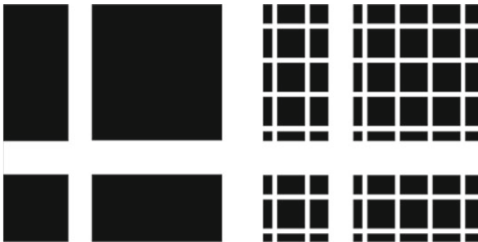
Fig. 1 Two levels of recursion of a Sierpinski carpet with fractal dimension D = 1.84 . The fracture pattern is perpendicular to the flow direction
