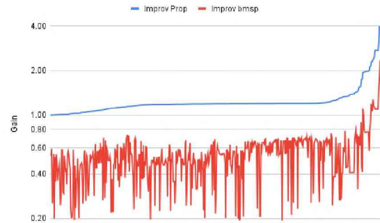
Figure 11: Factor of reduction when comparing the storage against CSR (i.e. size_{csr}/size_{optimized} and size_{csr}/size_{bmSparse} )
