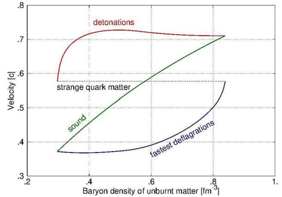
Figure 4: Velocity of the combustion front for detonations and the fastest deflagrations, and velocity of sound in baryonic matter. The velocity of the slowest deflagrations is zero. The first two curves also represent the velocity of the incoming baryonic matter with respect to the combustion front. The velocity of the outgoing strange quark matter is shown by the dashed segment.
