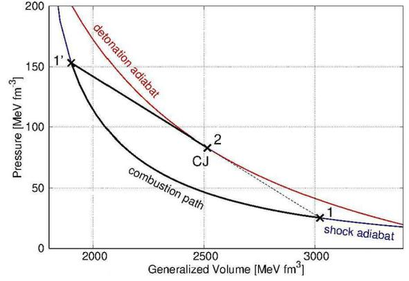
Figure 1: Shock adiabat, detonation adiabat and the path from initial state 1 to final state 2 for  $n_B = 0.35 \text{ fm}^{-3}$ . In this case the final state is the Chapman-Jouguet point.
