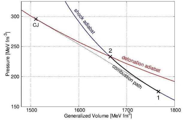
Figure 2: Shock adiabat, detonation adiabat and the path from initial state 1 to final state 2 for  $n_B = 0.75 \text{ fm}^{-3}$ . Here the final state is the crossing point between the adiabats.
