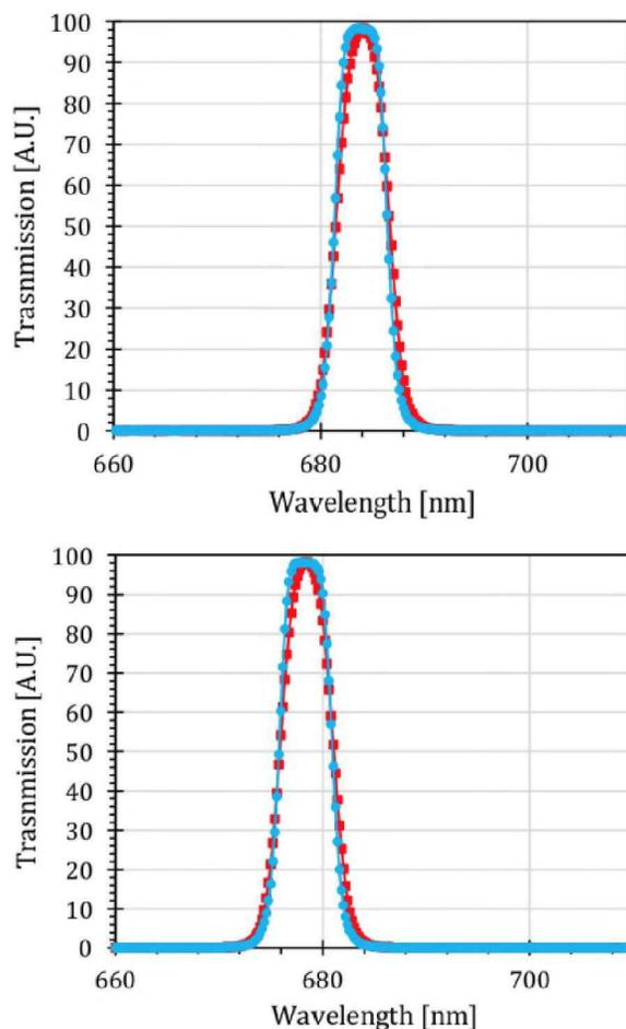
Figure 2: Transmission of the OVI - 683.5 nm (top) and OVIC - 678 nm (bottom) new filters, as measured at GS with the CARY 500 spectrometer (red), and as provided by the manufacturer (blue).
