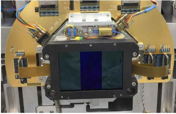
Figure 3: Photograph of the GMOS-N Hamamatsu focal plane array. The left- and right-most CCDs (CCDr and CCDb) are of type “BB”. The middle CCD (CCDg) is of type “HSC”. The golden semi-circular plate behind is the electrostatic discharge (ESD) protection board.
