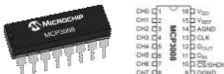
*Figura 11: Conversor ADC MCP 3008.*
