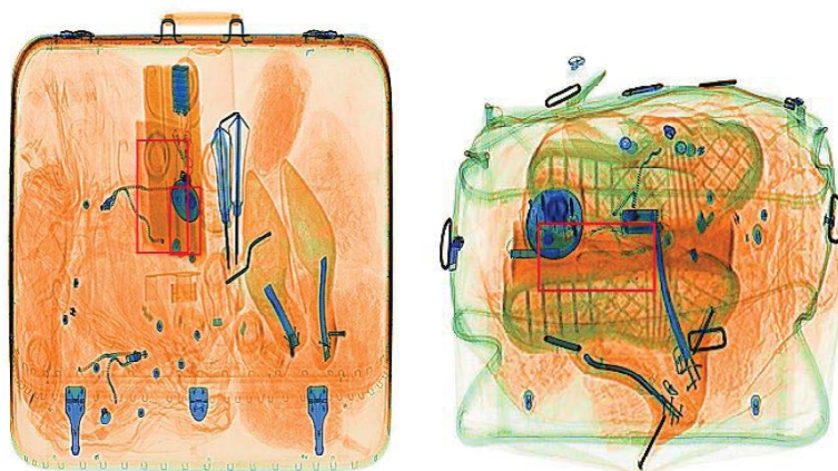
Fig. 2. Sample scanner image containing explosive artifacts composed of dynamite with a 9 volt battery (left) and TNT with AAA batteries (right). Both images belong to the “explosive” or “positive” class.
