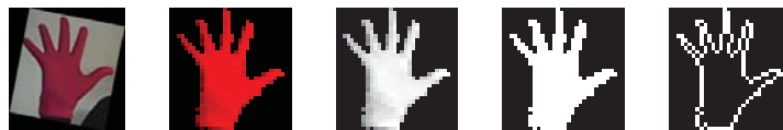
Fig. 6. From left to right: raw image, segmented image, grayscale image, hand segmentation mask, and contour.
