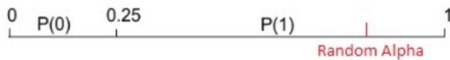
Figure 1. PAQ splits the [0,1) interval giving 1/4 of probability to bit 0 and 3/4 of probability to bit 1. When a random number is sampled in this context it is more likely to generate a 1. Each generated bit updates all models' context. However, that bit should not be learned because of its random nature. In other words, PAQ just learns from the training set and then generates random text using that probabilistic model. After 8 bits, a character is generated.
