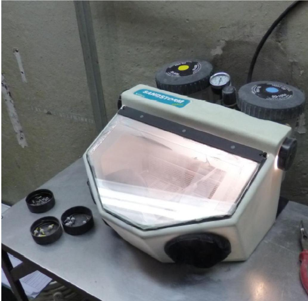
Figura 4.5: Granalladora Sand Storm, Vaiman. (Kinetical SRL, Berazategui, Argentina)
