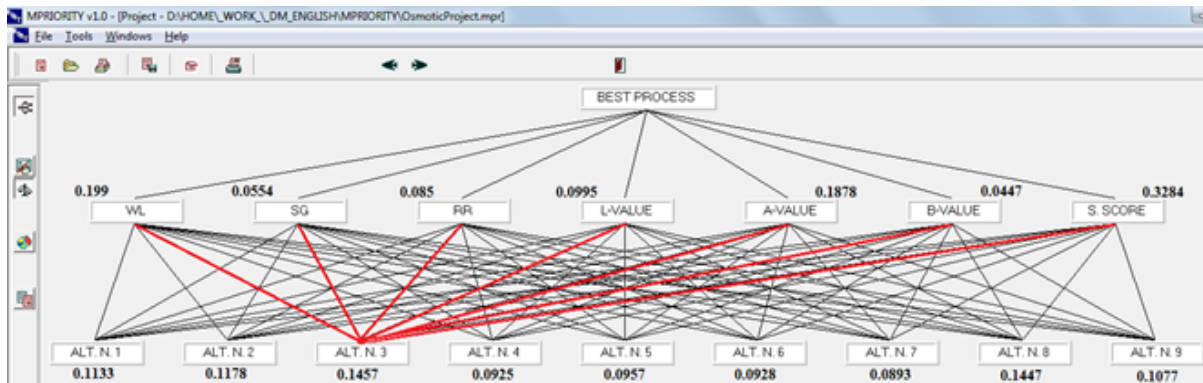
Figure 6: Hierarchy of decisions corresponding to the problem of choosing the most preferred osmotic dehydration process; the main goal (BEST_PROCESS) is set at the top of the hierarchy; the decision alternatives ALT.N.1-ALT.N.9 are at the bottom (see Table 10); the criterion of the decision problem (i.e. water loss (WL), solute gain (SG), rehydration ratio (RR), L-value, a-value, b-value, and sensory score(S.SCORE)) make up the middle of the hierarchy.
