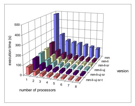
Figure 8 - Execution times for parallel matrix multiplication.
