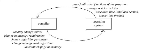
Figure 4 - Interaction between compiler and operating system under CAPR strategy.
