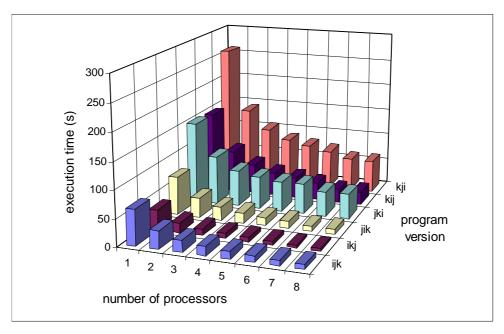
Figure 13 - Execution time for matrix multiplication program versions.
