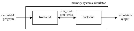
Figure 5 - Memory systems simulator internal structure.
